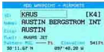
Once you bring up the Waypoint you are looking for, just press **CLEAR** or **MENU** to add it to the Flight Plan and the Waypoint will be inserted into the slot that was highlighted in the Flight Plan. When a Waypoint is added to the Flight Plan on the Moving Map, it is added to the end of the Flight Plan each time. In the Flight Plan window, the new Waypoint is inserted into the highlighted slot in the Flight Plan.
