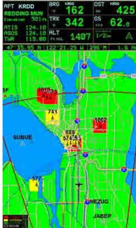
The AUTO setting for TAWS allows the EKP-IV to calculate the appropriate setting for you, based on the OCH. Once the OCH reaches 3,000 feet, the EKP-IV will switch to HIGH SEP, and in areas below an OCH of 3,000 feet the EKP-IV will operate in LOW SEP.
