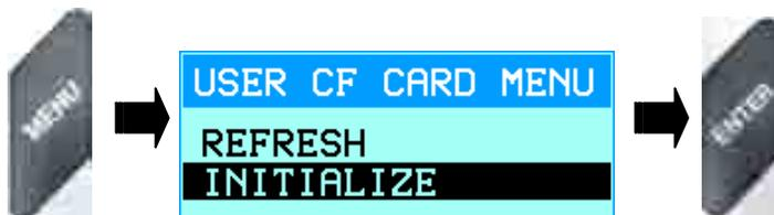
Once the CF card has been initialized, it is now ready for data storage. To save a file, press **ZOOM IN**, then enter the name in the space provided, press **ENTER** and select the type of file (Routes, Track, Waypoints) and then **ENTER** again to confirm.
