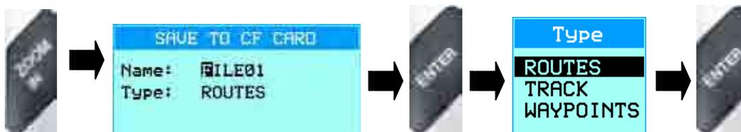
Conversely, highlighting a file and pressing **ZOOM OUT** will delete the file from the CF card. To load a file from the CF card, highlight it and press **ENTER**. The data will then be uploaded into the EKP-IV.
