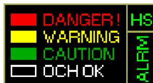
The red, yellow and green colors correspond to the Obstacle Clearance Height (OCH) at any given location. The OCH is calculated by subtracting the current elevation from your altitude. The shading varies in both the Highland and Lowland definitions accordingly:
