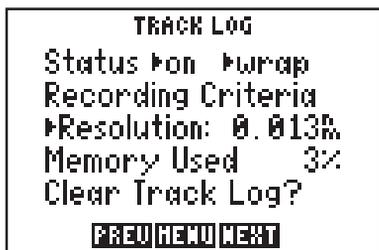
The Track Log Setup Page is used to configure the track log function. A track log is a record of your flight path showing where you have been up to your present position. The cyclic fields on line one allow you to turn the track storage on or off, and determine how the track log will be stored in memory.
