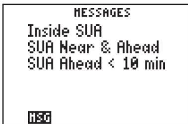
The GPS 95 provides four different SUA messages (alerts) depending on your location relative to a special-use airspace. These SUA messages are only given when the SUA alarms are on and when your ground speed exceeds 30 knots. (See Section 8.10 for more information on SUA alarms.)
