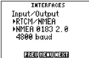
The GPS 95 can use Differential GPS (DGPS) corrections in RTCM SC-104 version 2.0 format. DGPS corrections in this format can be received from an external device (capable of output in 6 to 8 byte format as specified by RTCM SC-104 version 2.0) by connecting the device to the input port on the back of
