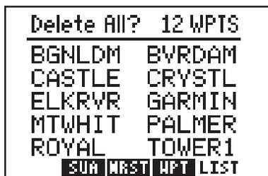
The Waypoint List Page allows you to view all stored user waypoints in your GPS 95. The list may be scrolled, with the arrow keys, to view all the waypoints. From this page, waypoints may be selected for deletion, renaming or to activate a GOTO. (See Chapter 4 for information on the GOTO function.)
