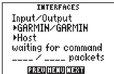
A second cyclic field also appears when the GARMIN input/output is selected. The GARMIN option allows you to exchange data such as waypoints, routes, track logs and satellite almanac data with another GPS 95 or with a PC-compatible computer. You may select between
