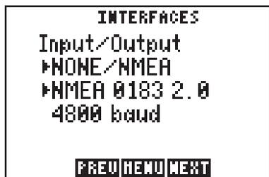
From the Input/Output Page, you may select the input and/or output format needed to connect your GPS 95 to other equipment: PC, NMEA device, etc. You may select no input/output (NONE/NONE), GARMIN input/output (GARMIN/GARMIN), NMEA output (NONE/NMEA), RTCM input/NMEA output (RTCM/NMEA) or RTCM input (RTCM/NONE).
