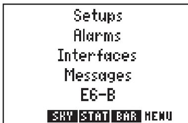
The GPS 95's menu pages allow you to do setup functions to customize your unit and E6-B calculations to plan your flight. The Main Menu lets you select from five functional categories: Setups, Alarms, Interfaces, Messages and E6-B calculations. Selecting “Messages” lets you view the Message Page. Selecting one of the other items
