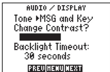
From the Audio/Display Page you can turn the message and/or keypad tones on and off, change the display contrast and change the time-out for the display backlighting.
