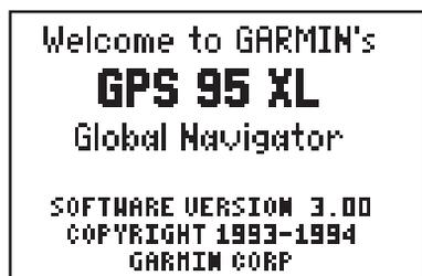
Turn the GPS 95 on. The unit will display the welcome screen and perform several diagnostic checks to ensure that proper operation will occur.
